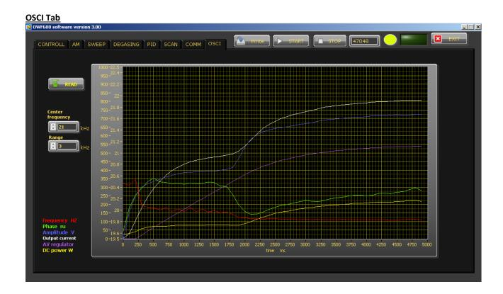
Go back to the first tab - CONTROL. Play with different values of MMM and AMMM parameters (but very slowly and carefully) for improving better results. If OVERCURRENT occurs, than you overvalued the MMM and/or AMMM parameters.
