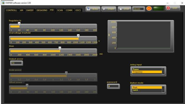
**Regulator**  $k_i$  – This an integral constant of the internal PID regulator. Use this to adjust the response time of the regulator. When  $k_i$  is low – the response time is high(the regulator is slow), when  $k_i$  is high – the response time is low(the regulator is fast).
