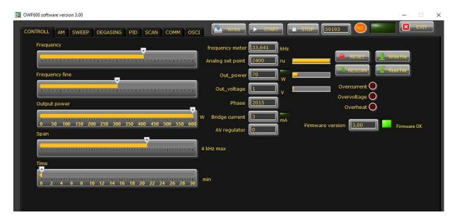
Set frequency little bit higher (+500 Hz), than frequency of ultrasonic transducers is. Keep other parameters as presented on the picture below, but In the very first start here are the steps and settings:
